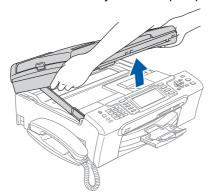
Insert the network cable into the LAN socket marked with a R symbol. You will find the LAN socket inside the machine on the left as shown below.
